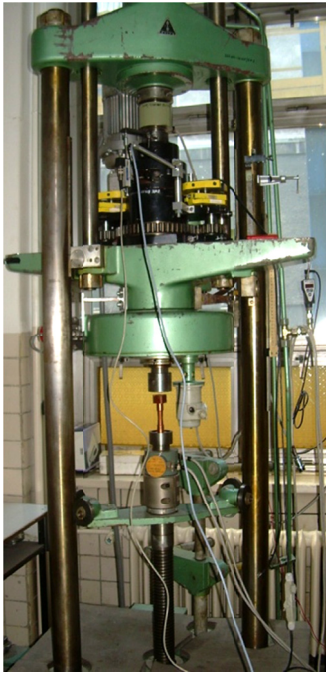
Fig. 1. Universal machine for testing materials under complex loading conditions
