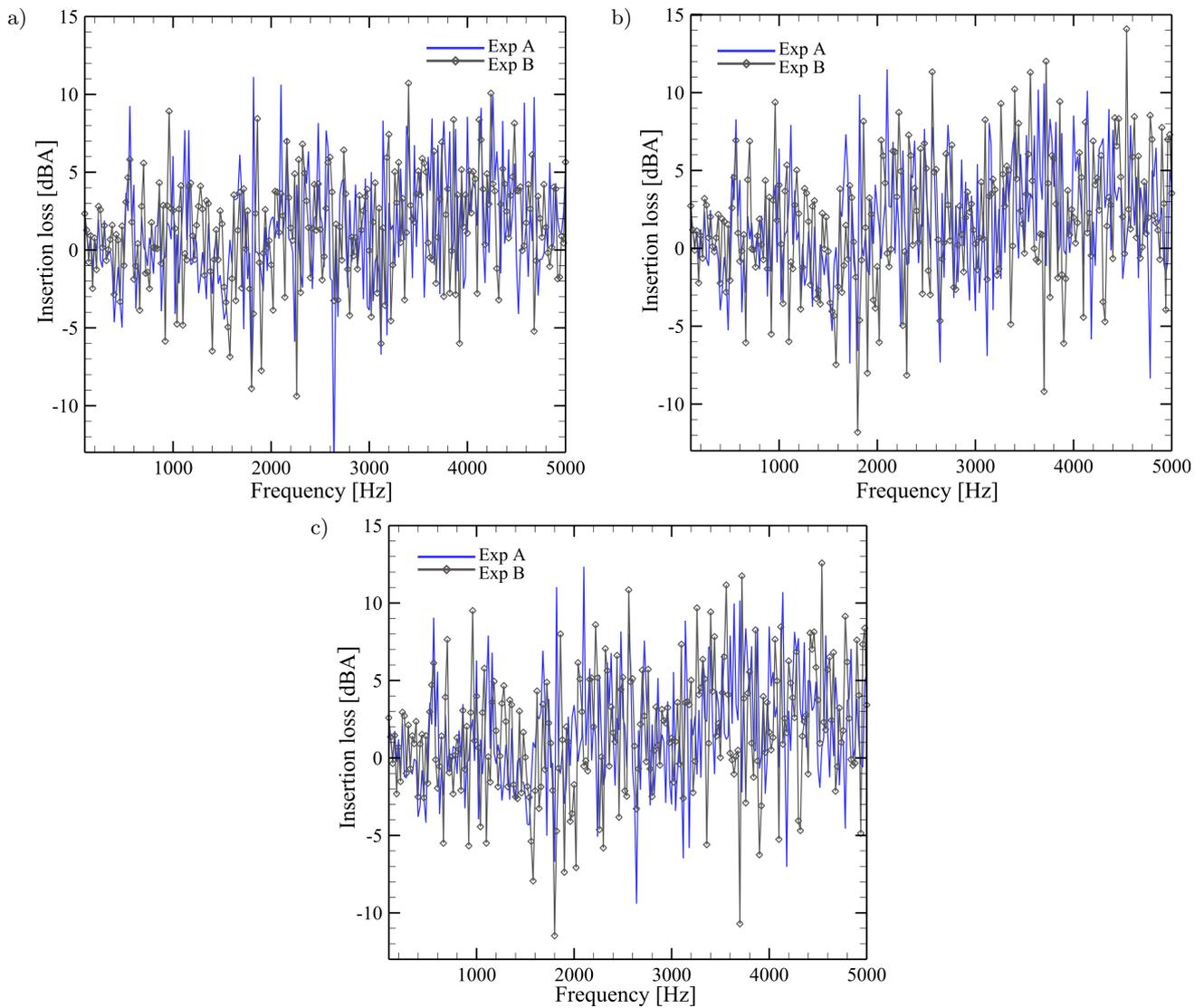
Fig. 4.  $IL_2$  obtained by the plenum window with HRs (attached 90° jagged flap) when comparing with the case of without resonators for experiments A and B: a) white noise, b) traffic noise, c) construction noise.
