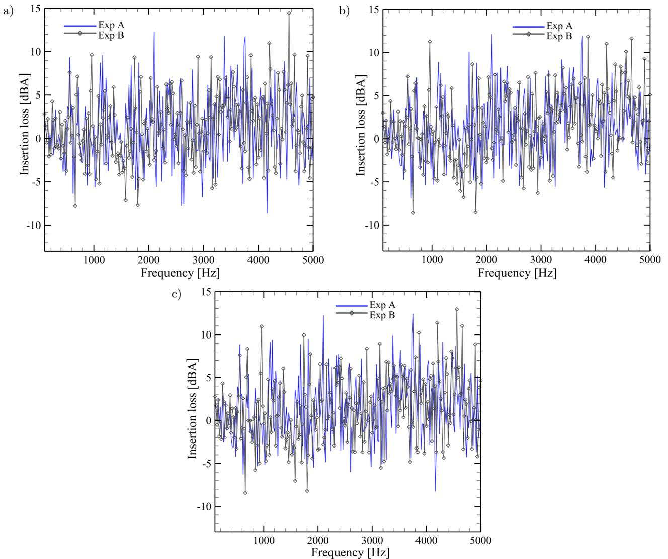
Fig. 3.  $IL_2$  obtained by the plenum window with HRs (without jagged flap) when comparing with the case of without resonators for experiments A and B: a) white noise, b) traffic noise, c) construction noise (the data are recorded at interval of 2 Hz, but the results are presented at interval of 20 Hz for clearer presentation of the IL trends).
