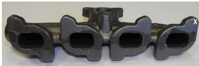
Fig. 1. Exhaust manifold made of SiMo iron; X –location of the sample for microstructure examination
