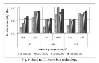
The hot strength of Sands no II, III, IV was 0.43 - 0.93 MPa after 30 seconds of curing, 0.77 - 1.62 MPa after 60 seconds of curing, 1.02 - 1.73 MPa after 90 seconds of curing and 1.06 - 2.04 MPa after 120 seconds of curing, and it depended on the core box temperature and binder content.
