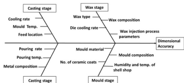
Fig. 2. Factors affecting dimensional accuracy of IC process
