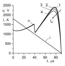
Fig. 4. Current *i* and voltage *u* curves in a circuit with the arc model (39) during circuit interruption ( $P_M = 2.2 \text{ MW}$ ,  $\tau = 9 \text{ µs}$ ,  $\cot \psi = 386.1 \text{ V/µs}$ ,  $U_{cr} = 1250 \text{ V}$ ,  $i_{cr} = 1000 \text{ A}$ ,  $\beta = 4.683 \cdot 10^{-3} \text{ A}^{-2}$ ,  $G_0 = 1.5 \text{ S}$ ) with various residual currents in the model ( $1 - I_M = 0 \text{ A}$ ,  $2 - I_M = 50 \text{ A}$ ,  $3 - I_M = 100 \text{ A}$ ,  $4 - I_M = 150 \text{ A}$ )
