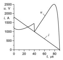
Fig. 5. Current and voltage curves in a circuit with the arc model (23) during circuit interruption ( $P_M = 2 \text{ MW}$ ,  $\tau = 8 \text{ }\mu\text{s}$ ,  $\cot \psi = 800 \text{ V}/\mu\text{s}$ ,  $U_{cr} = 1250 \text{ V}$ ,  $i_{cr} = 1000 \text{ A}$ ,  $\Delta U = 500 \text{ V}$ ,  $G_0 = 1.5 \text{ S}$ ,  $I_M = 10 \text{ A}$ )
