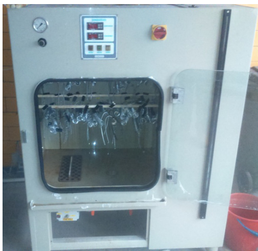
Fig. 5. The CORROTHERM Model 610 salt spray chamber
