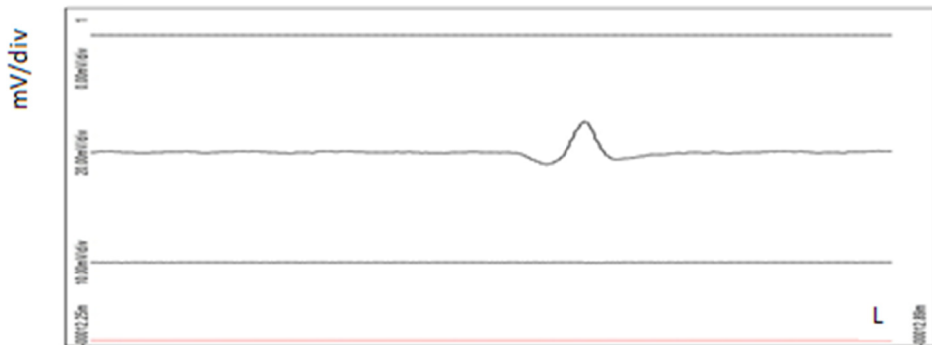
Fig. 11. Image of the damage No. 4 by the classic magnetic method
