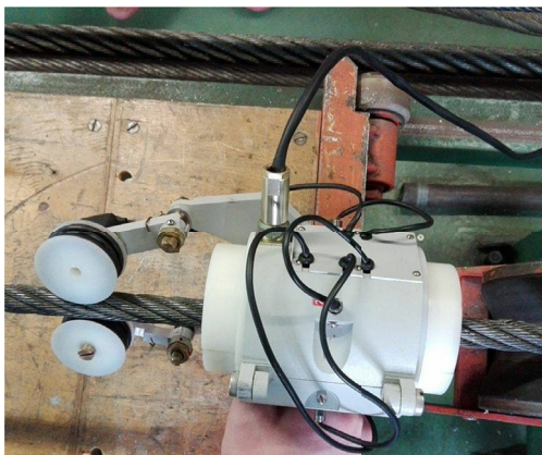
Fig. 2. Measuring head for testing ropes
