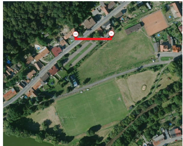
Fig. 7. Distance between RF generator and receiver 58 m
