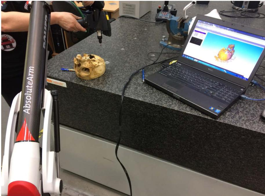
Fig. 2. A procedure for making a skull reference model
