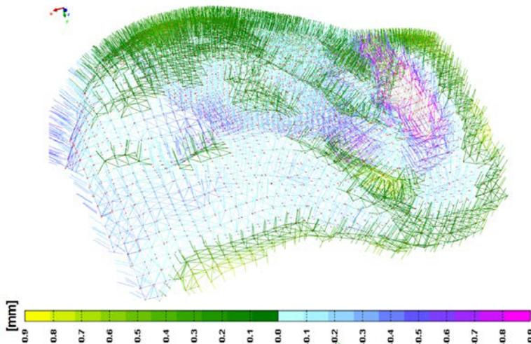
Fig. 11. Vectors of imaging precision errors for the cranium specimen from the zygomatic bone in the tomographic model vs., reference model
