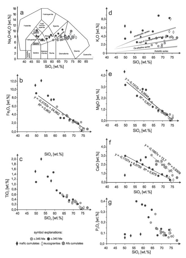
Text-fig. 5. Major elements versus SiO<sub>2</sub> variation diagrams of High Tatra granitoids, including TAS discrimination diagram after Middlemost (1985) (a) and the K<sub>2</sub>O versus SiO<sub>2</sub> diagram after Peccerillo and Taylor (1976) (d)
