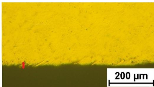
Fig. 22. The image of the surface layer of CuZn37As0.37 alloy.
