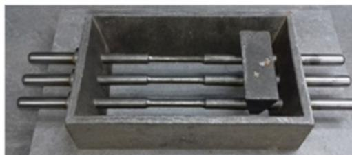
Fig. 3. The set-up for making sand moulds
