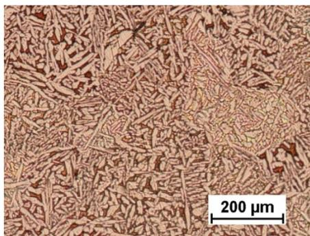
Fig. 9. The microstructure of MS-60 alloy, the casting from the metal mould obtained from the charge in the form of ingots
