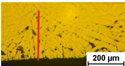
Fig. 17. The image of the surface layer of CuZn37Al1.21 alloy.
