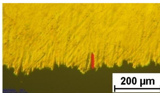
Fig. 21. The image of the surface layer of CuZn37As0.055 alloy.
