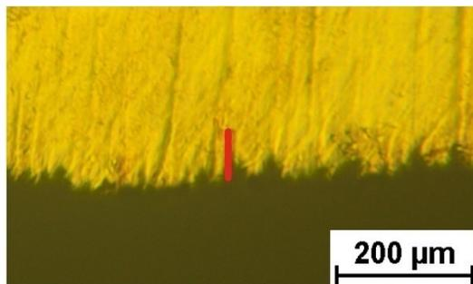
Fig. 20. The image of the surface layer of CuZn37As0.033 alloy.
