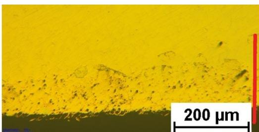
Fig. 18. The image of the surface layer of CuZn37Sn0.71 alloy.
