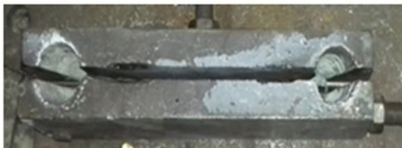
Fig. 6. A divided metal mould
