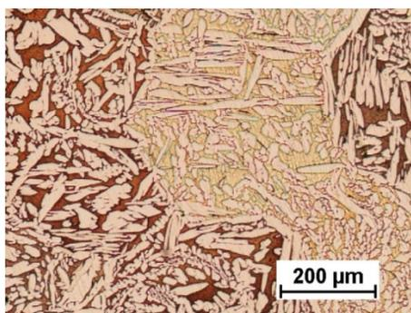
Fig. 8. The microstructure of MS-60 alloy, the casting from the OBB Sand mould obtained from the charge in the form of ingots
