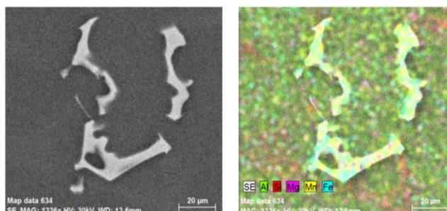
Fig. 2. Mapping of skeletal particle Al<sub>15</sub>(FeMn)<sub>3</sub>Si<sub>2</sub> phase of the secondary A4 alloy a) SEM b) Mapping
