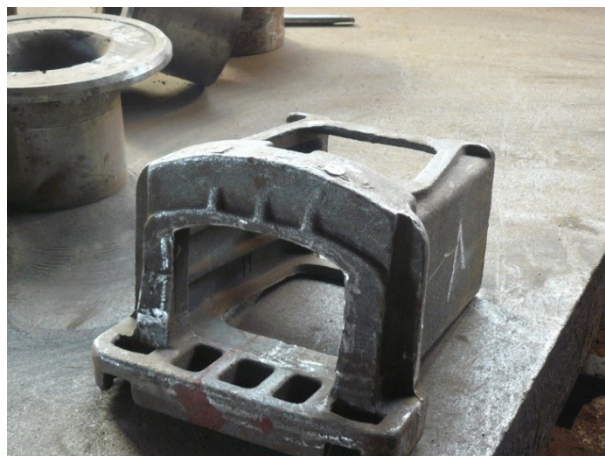
Fig. 4. Appearance of the casting "Front Buffer Stop" obtained using a liquid glass mixture with softening additive
