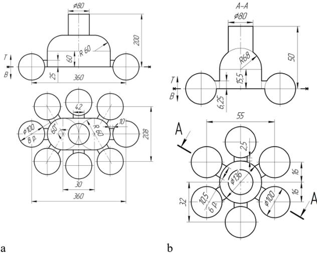
Fig. 1. Diagrams of sprue and supply systems for casting spherical grinding bodies into a sand mold with a horizontal joint
