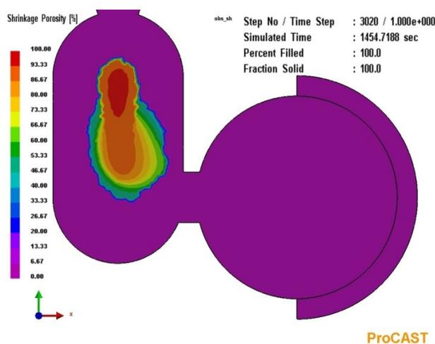
Fig. 9. Porosity distribution in casting over the section
