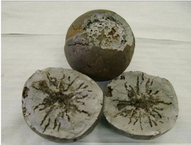
Fig. 4. Shrinkage and gas defects in castings of grinding bodies
