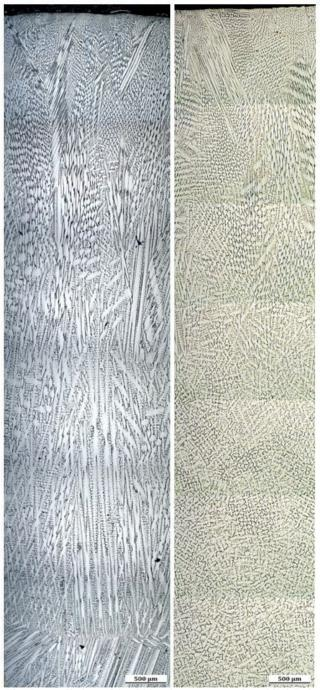
Fig. 4 Overall view of dendritic microstructure of Co-20Ni-7Al-7W alloy on the transverse (left) and longitudinal (right) section
