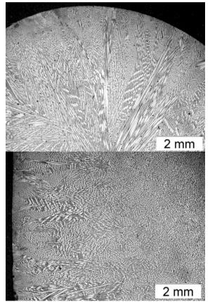
Fig. 3 View of dendritic microstructure of Co-20Ni-7Al-7W alloy on the transverse (up) and longitudinal (down) section
