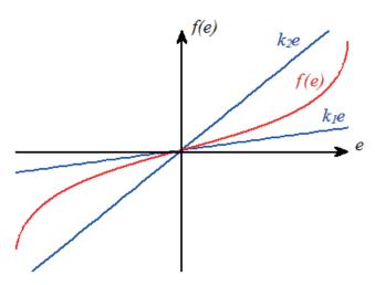
Fig. 2. Characteristic of nonlinear element
