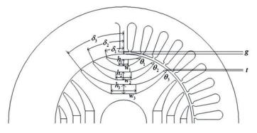
Fig. 2. Parametric model of a PMASR motor section
