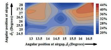
Fig. 9. Influence of change of  $\delta_1$  and  $\delta_2$  of PMASR motor on torque ripple percentage
