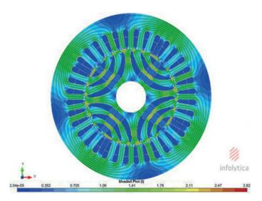
Fig. 5 Magnetic flux density distribution of a PMASR motor at rated operating conditions
