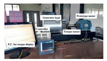
Fig. 6. Experimental test setup
