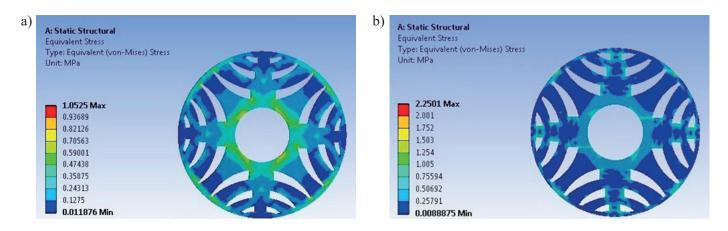
Fig. 15. Von Mises stress distribution of (a) design solution 1 (b) design solution 2 of PMASR motor
