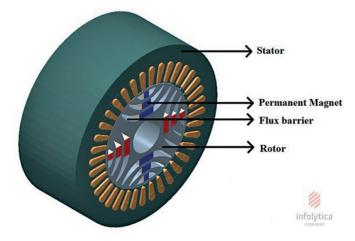
Fig. 1. 3D Model of PMASR motor
