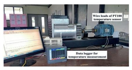
Fig. 11. Experimental setup for estimation of stator core and winding temperature
