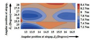
Fig. 8. Influence of change of  $\delta_1$  and  $\delta_2$  of PMASR notor on average torque
