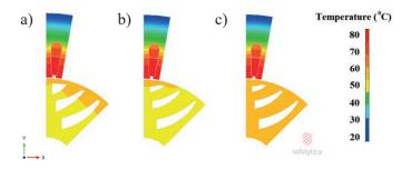
Fig. 14. Comparison of temperature distribution for different parts of 1/8<sup>th</sup> cross section of PMASR motor (a) prototype (b) design solution 1 and (c) design solution 2
