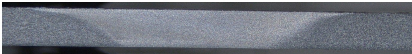
Fig. 9. Transverse view of a weld made with a carbide tool WT1 joint of AA 2024 T3 sheet of 1 mm thickness using carbide tool with smooth shoulder at 2000 rpm and welding speed 200 mm/min (No. 2)
