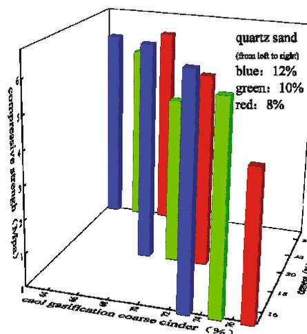
**Fig. 1.** The compressive strength of the non-sintered ceramsite
