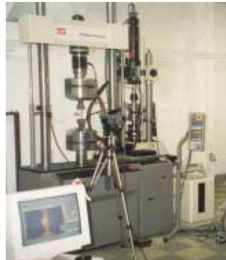
Fig. 1. Scheme and photograph of the experimental set-up designed for thermomechanical investigation of the stress induced phase transformations in shape memory alloys
