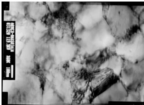
Fig. 29. TEM image of the Fe microstructure after Max Strain process
