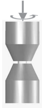
Fig. 3. Scheme of the HPT process
