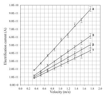
Fig. 2. Electrification current of insulating liquids vs. flow velocity through a metallic pipe: 1 – fresh mineral oil, 2 – synthetic Midel 7131, 3 – natural Midel 1204, 4 – aged mineral oil
