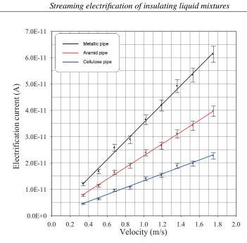
Fig. 3. Electrification current vs. flow velocity of natural ester Midel 1204 through the pipes made of various materials
