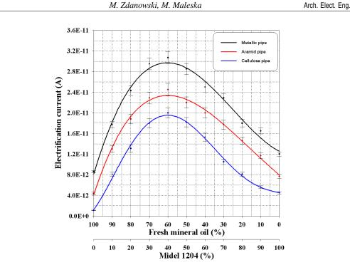
Fig. 5. Electrification current vs. percent content of natural ester Midel 1204 and fresh mineral oil in the mixtures
