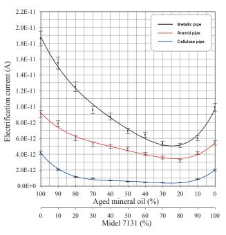
Fig. 6. Electrification current vs. percent content of synthetic ester Midel 7131 and aged mineral oil in the mixtures
