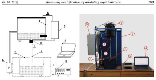
Fig. 1. Layout of the test stand with a flow pipe for testing streaming electrification of insulating fluids:
