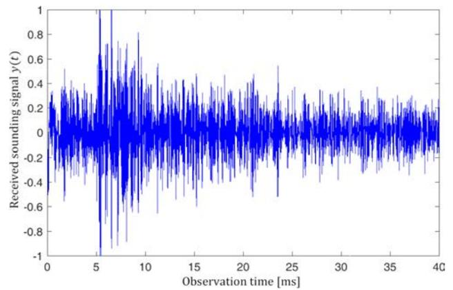
Fig. 9. A sequence of received pulses if the narrow signal pulse is transmitted with a period of transmitting of 40 ms.
