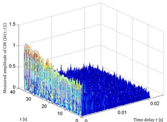
Fig. 6. The amplitude of the CIR measured in Thongnhat lake in a condition of quasi-static environment.
