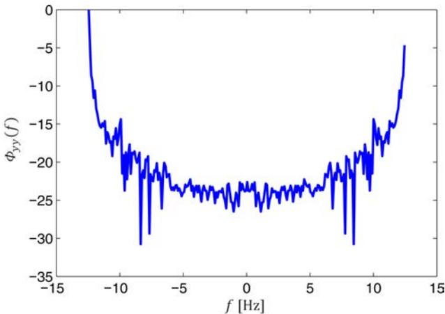
Fig. 12. The Doppler spectrum of the underwater acoustic channel.
