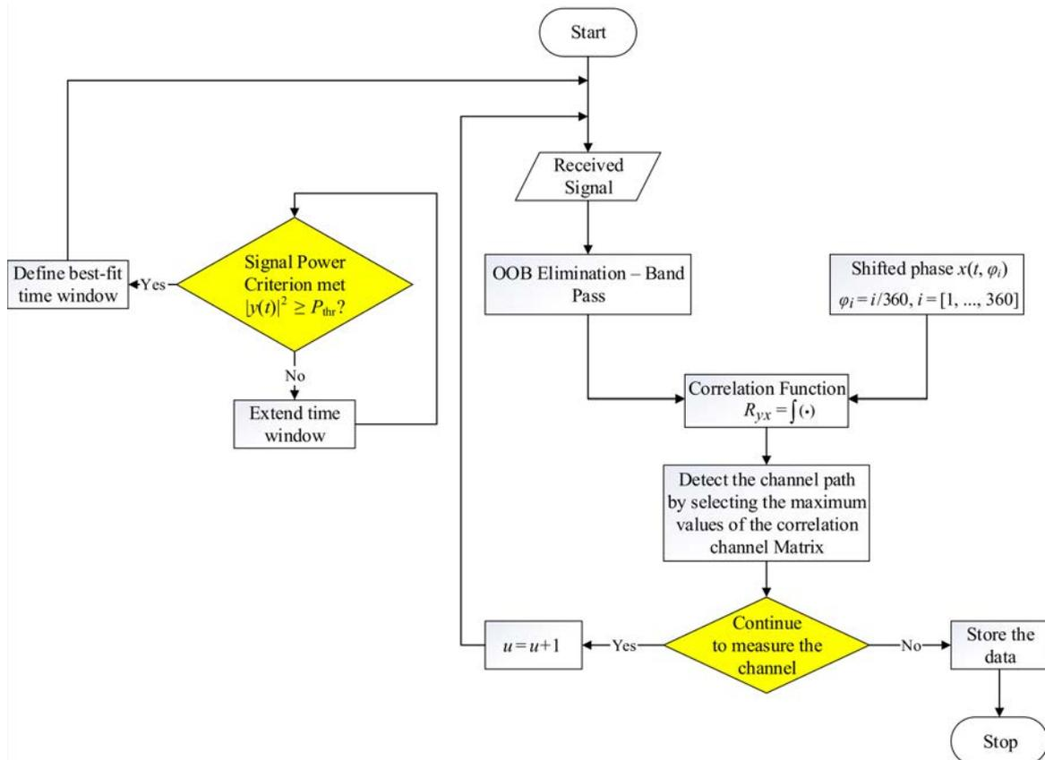
Fig. 2. Best-fit time windowing method combined with correlation for maximum PDP and Doppler detection.
