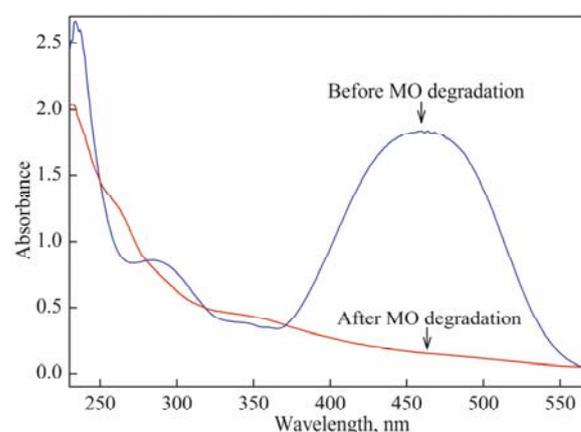
Fig. 6. Change of UV/Visible adsorption spectra with reaction time in BES
