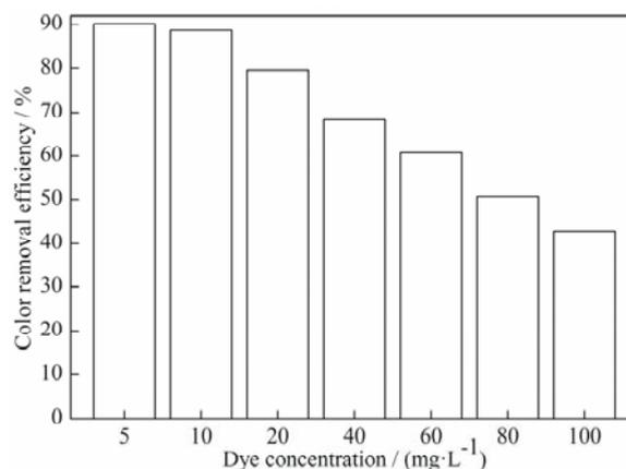
**Fig. 3.** Color removal efficiency with different dye concentration of influent in BES
