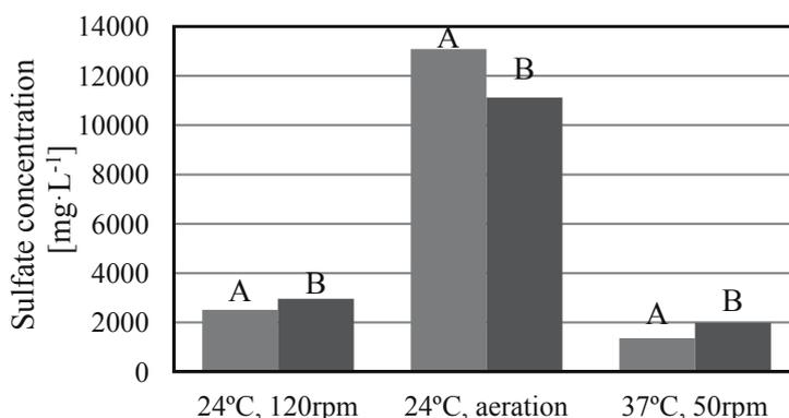
Fig. 9. Sulfate concentration in various variants of leaching culture after 5 days of bioleaching [ $\text{mg}\cdot\text{L}^{-1}$ ]
