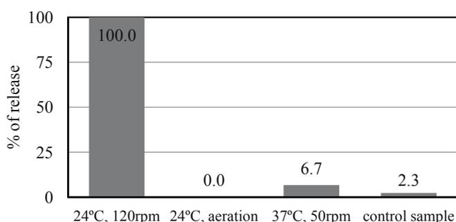
Fig. 3. Efficiency of niobium release from ash sample A
