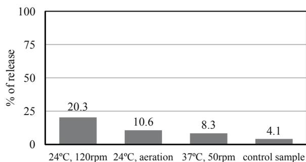
Fig. 6. Efficiency of rhodium release from ash sample B
