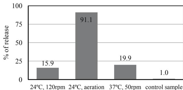
Fig. 2. Efficiency of cadmium release from ash sample A
