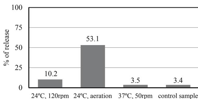
Fig. 8. Effectivity of indium release from ash sample B
