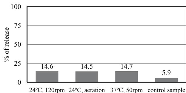
Fig. 7. Effectivity of niobium release from ash sample B
