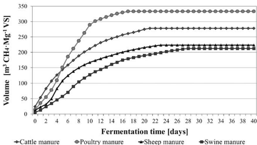
**Fig. 4.** BMP assay curves showing cumulated methane production (Nm<sup>3</sup>CH<sub>4</sub>·Mg<sup>-1</sup> VS) from 4 different substrates (CM, PM, SHM and SWM). Source: developed by authors
