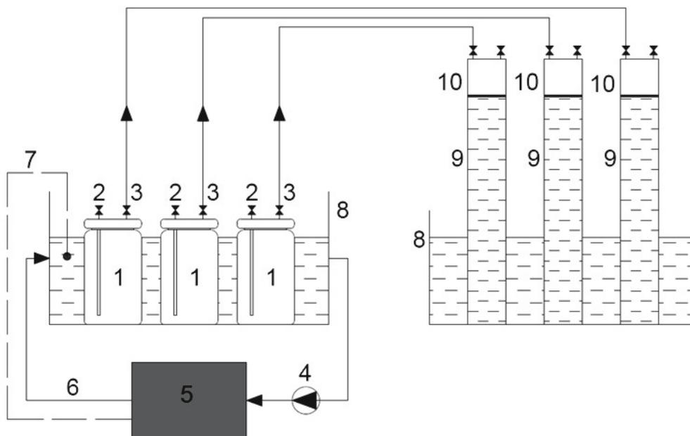
**Fig. 3.** Scheme of the AD reactors in BMP test (1. Biofermenter with the input of 1.8 dm<sup>3</sup> of capacity, 2. Sampling tube, 3. Tube for biogas flow, 4. Water pump, 5. Water heater with a temperature in the range of 20–70°C, 6. Isolated hot liquid tube, 7. Temperature sensor, 8. Reservoir, 9. Biogas container made of poly (methyl methacrylate), 10. Liquid barrier).
