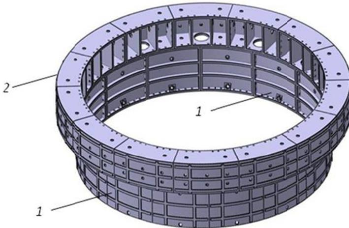
Fig. 11. Illustration of the tubing lining's load bearing column.
