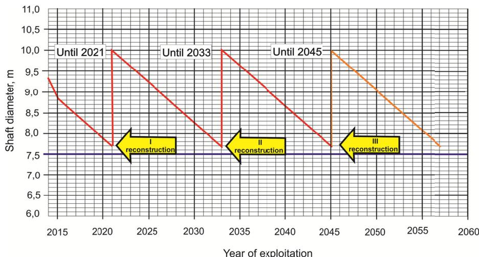
Fig. 8. Hypothetical plan for SW-4 shaft reconstructions along the salt rock section (based on Fabich et al., 2016)
