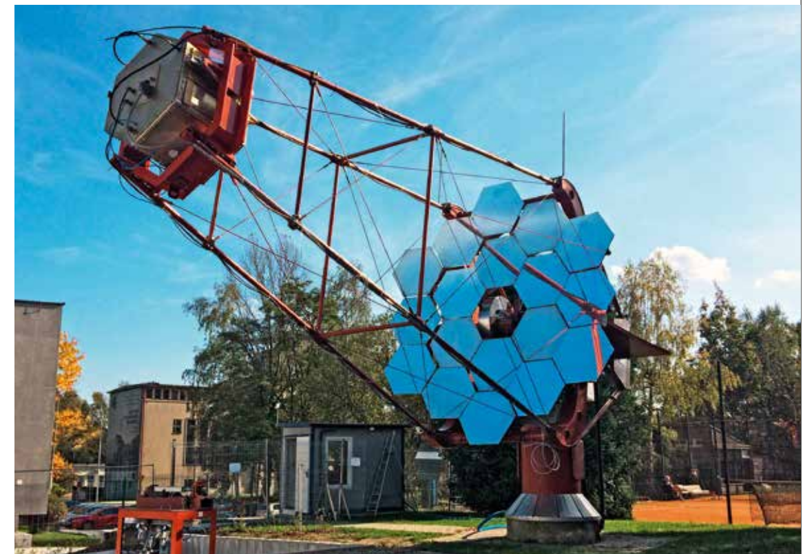
Prototype of the SST-1M telescope with camera mounted at the PAS Institute of Nuclear Physics in Kraków. The telescope has a diameter of 4 m. It comprises 18 spherical mirrors. The focal length is 5.6 m and the field of vision is 9.1 degrees.
