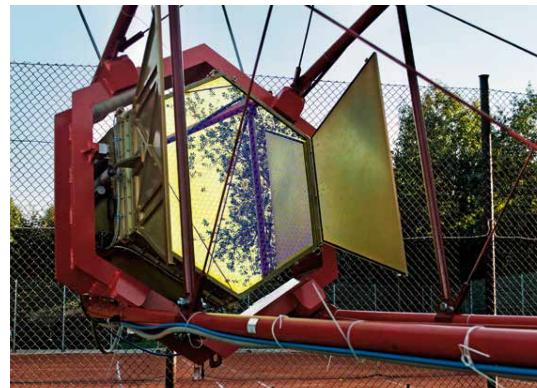
Camera of the SST-1M prototype telescope before sunrise and the closure of the cover.
