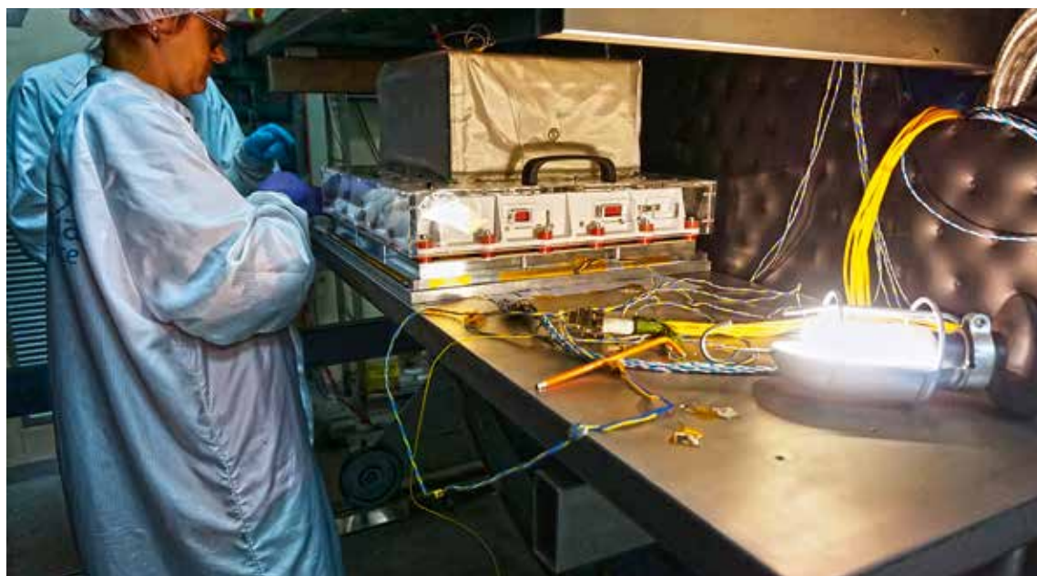
The POLAR detector undergoing thermal tests at the laboratory in Terni, Italy.
