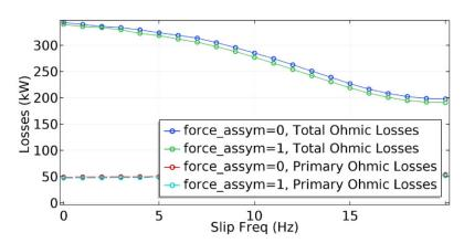
Fig. 15. Comparison of total losses and primary losses in the subject LIM for the symmetrical and unsymmetrical supply (v = 30 m/s)
