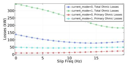
Fig. 9. Comparison of total losses and primary losses in the subject LIM for differrent supply modes ( $\nu = 30$  m/s)
