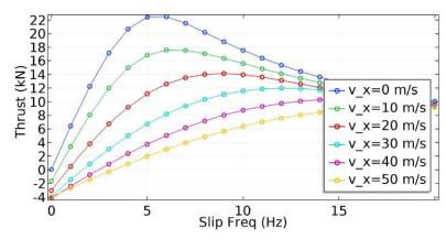
Fig. 10. LIM characteristics obtained for the current-supply (I = 550 A)
