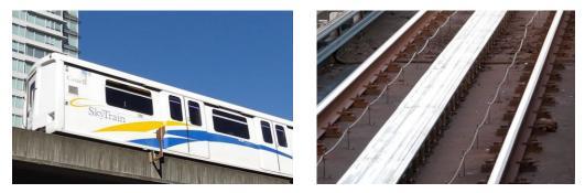
Fig. 1. SkyTrain car (left) and its reaction rail (right)
