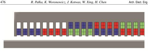
Fig. 2. End part of the LIM showing geometric assymetry and the asymmetric phase windings distribution
