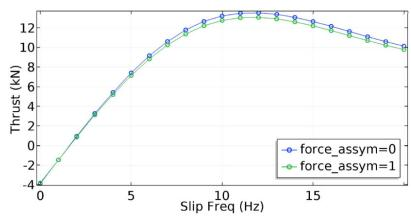
Fig. 13. LIM characteristics obtained for the symmetrical (I = 550 A in all phases) and unsymmetrical supply ( $I_1 = 550$  A,  $I_2 = 540$  A,  $I_3 = 530$  A) for the speed v = 30 m/s
