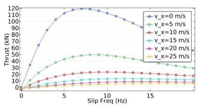
Fig. 11. LIM characteristics obtained for the voltage-supply (V = 460 V)
