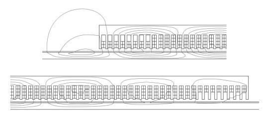
Fig. 3. Magnetic field distribution within the LIM
