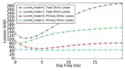
Fig. 6. Comparison of total losses and primary losses in the subject LIM for differrent supply modes ( $\nu = 10$  m/s)
