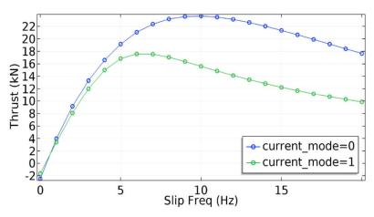
Fig. 4. Comparison of thrust values for both supply modes (v = 10 m/s, current mode: I = 550 A, voltage mode: V = 460 V)
