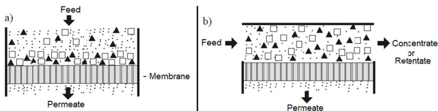
Fig. 6. a) Dead-end flow filtration scheme b) cross flow filtration scheme (Narebska, 1997)
