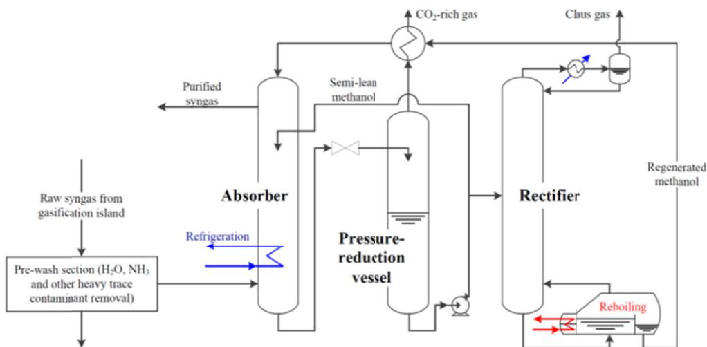
Fig. 3. Lurgi patented Rectisol<sup>®</sup> (Gatti et al., 2015)
