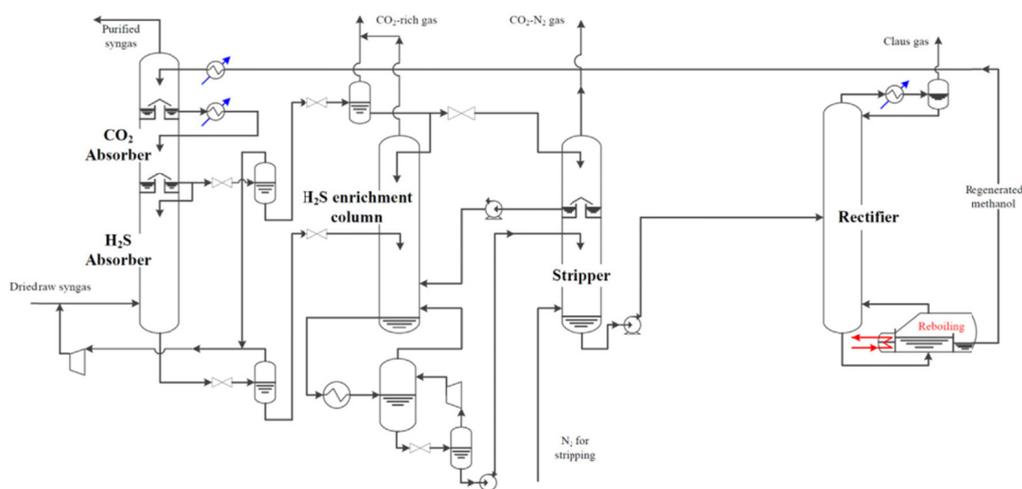
Fig. 4. Linde patented Rectisol (Gatti et al., 2015)
