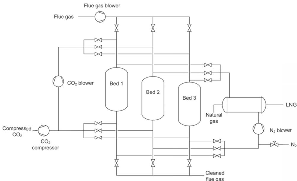
Fig. 9. Simplified process scheme for cryogenic CO<sub>2</sub> capture (Tuinier et al., 2011)
