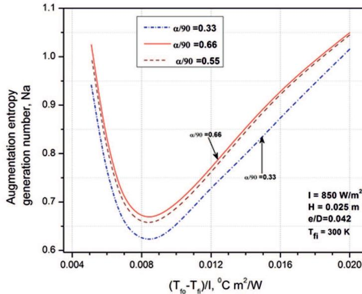
Figure 10: Variation of augmentation entropy generation number ( $Na$ ) with temperature rise parameter  $(T_{fo}-T_{fi})/I$  for different values of  $\alpha/90$ .
