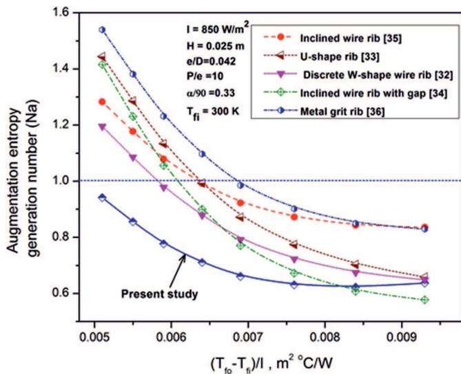
Figure 12: Comparison of augmentation entropy generation number (Na) of arc-shape wire roughness geometry with other roughness geometries of roughened SAH duct in lower range temperature rise parameter below  $0.010 \text{ } ^\circ\text{C m}^2/\text{W}$ .
