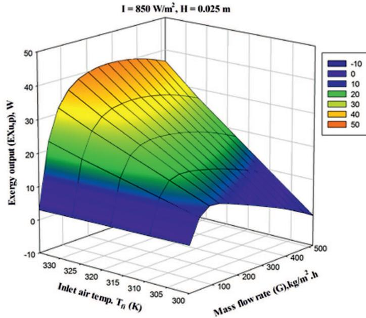
Figure 6: Variation of exergy output rate ( $EX_{u,p}$ ) with mass flow rate ( $G$ ) and inlet air temperature ( $T_{fi}$ ).
