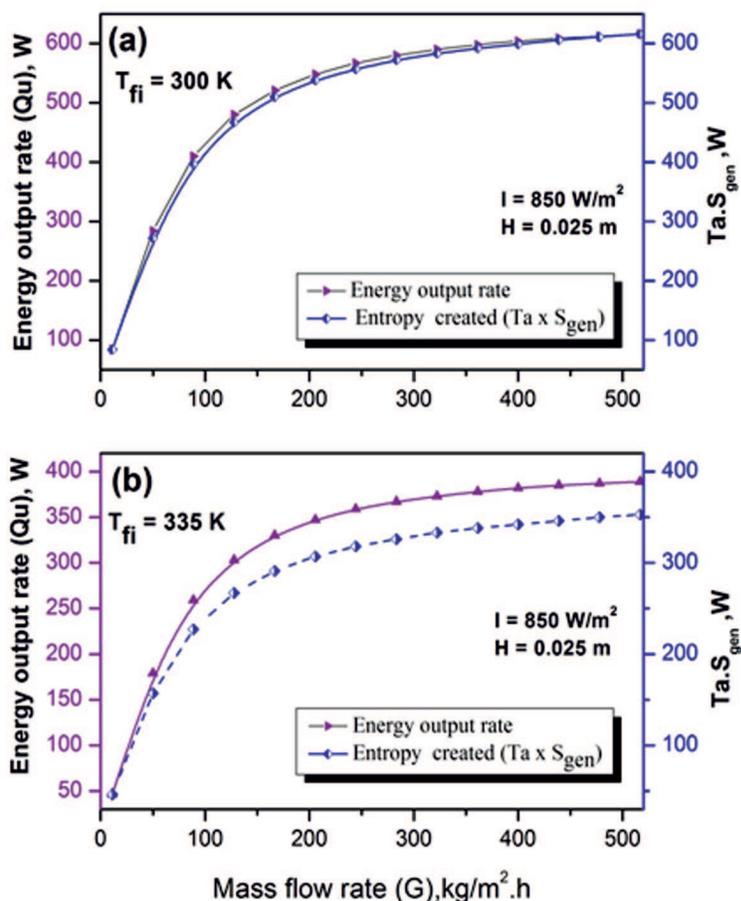
Figure 4: Variation of energy output rate ( $Q_u$ ) and entropy created ( $T_a S_{gen}$ ) with mass flow rate ( $G$ ): (a) at  $T_{fi} = 300$  K, (b) at  $T_{fi} = 335$  K.
