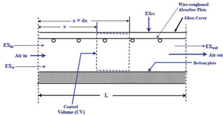
Figure 3: Control volume of exergy analysis of SAH.
