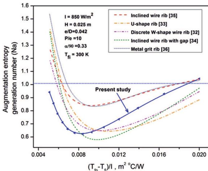
Figure 11: Comparison of augmentation entropy generation number (Na) of arc-shape wire roughness geometry with other roughness geometries of roughened SAH duct.
