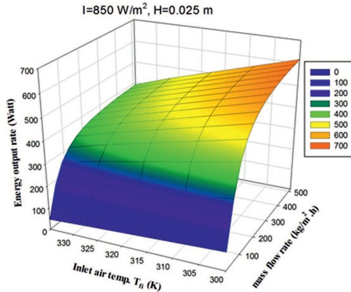
Figure 7: Variation of energy output rate ( $Q_u$ ) with mass flow rate ( $G$ ) and inlet air temperature ( $T_{fi}$ ).
