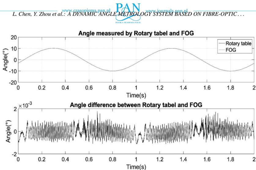
Fig. 4. Angle measured by two sensors under amplitude =  $10^\circ$ , frequency = 1 Hz sway movement.
