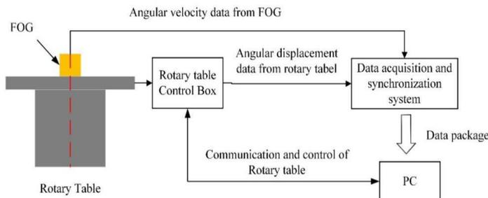
Fig. 1. Schematic of dynamic angle metrology system.
