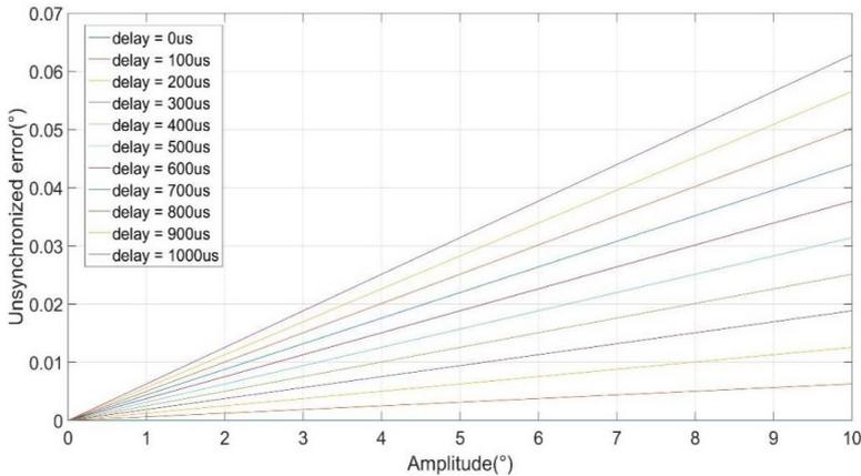
Fig. 2. Effect of amplitude and delay on non-synchronization error.
