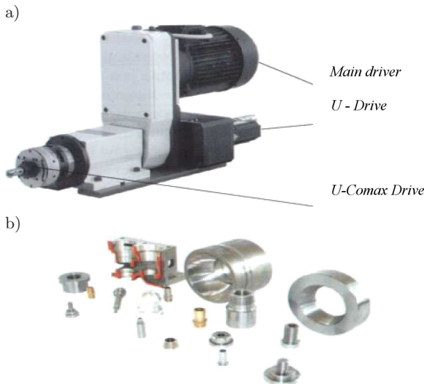
Fig. 13. U-COMAX head with independent drives (a) and examples of products made with it (b) [D'Andrea solution [37]].
