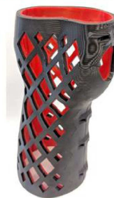
Fig. 11. Examples of products printed with the use of FDM (Rapid Prototyping Laboratory at Poznan University of Technology).
