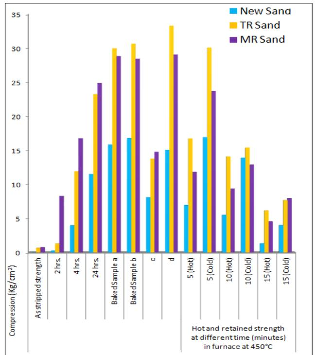
Fig. 11. Recipe: 0.8:50 Medium Fast Catalyst RT-20°C, RH-47%
