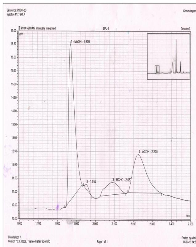
Fig. 3. GC of liquid portion of mass released on gelation of Resin and Hardener 100:20 (W/W)
