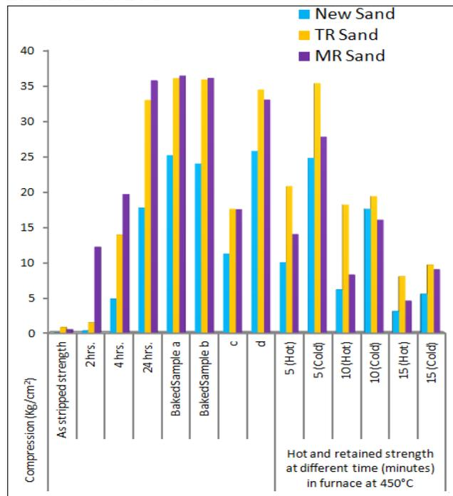
Fig. 10. Recipe: 1.0:50 Medium Fast Catalyst RT-20°C, RH-47%
