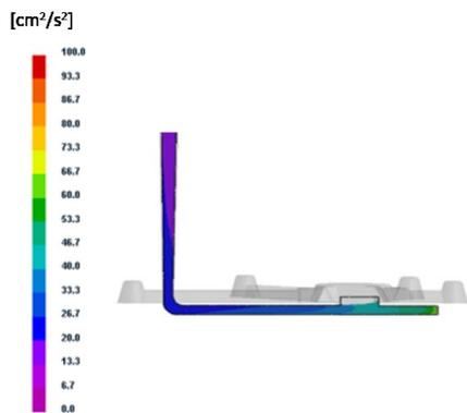
Fig. 5. Turbulence of melt – naturally pressurized gating system
