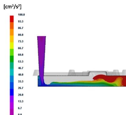
Fig. 3. Turbulence of melt – non-pressurized gating systems
