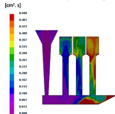
Fig. 8. Oxide occurrence - non-pressurized gating systems with chamfer
