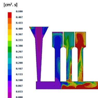
Fig. 7. Oxide occurrence - non-pressurized gating systems
