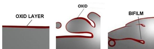
Fig. 1. Process of creation of bifilm
