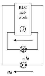
Fig. 1. The complex network with multicurrent power; i – internal mesh currents vector;  $i_0$  external current vector
