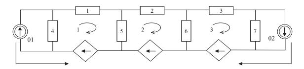
Fig. 3. A ladder system powered from two sides and optimal control sources distributed in the meshes of the ladder circuit
