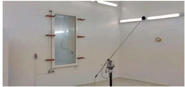
Fig. 1. View of the receiving room along with the measuring hole in the laboratory at AGH University of Science and Technology in Kraków.
