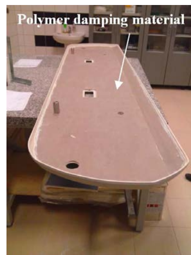
Fig. 10. Laminate bogie cover.
