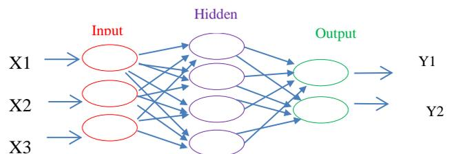
Fig. 2. A feed-forward network with one hidden layer [17]
