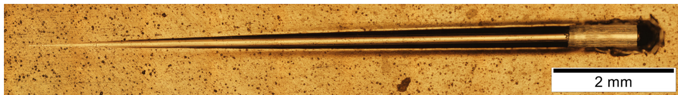
Fig. 12. Scratch test result for the LSA + SDS coating
