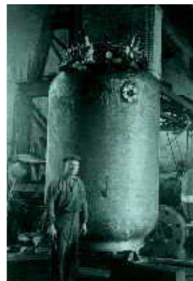
Fig. 1. Protocol from 1930 describing the study of duplex stainless steel grade 453S with 25% Cr, 1.5% Mo (left side), gunpowder reactor of the same steel grade supplied to a Belgian factory in 1933 (right side) [11]
