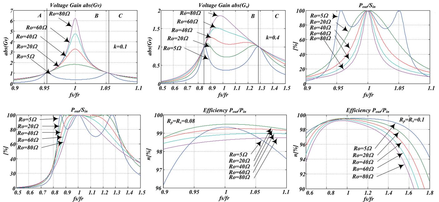
Fig. 5. Frequency characteristics of magnetic coupled coils with S-S compensation circuit for magnetic coupling factor  $k = 0.1$  and  $k = 0.4$  and load resistance  $R_o$  as parameter
