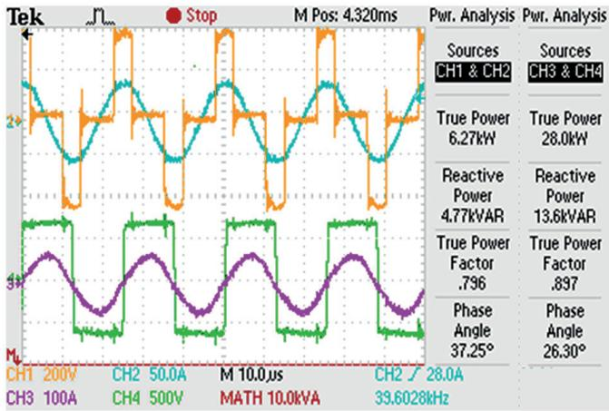
Fig. 12. Currents ( $i_p$  – CH1 scale: x1,  $i_s$  – CH3 scale /5) and voltages ( $u_p$  – CH2 scale: x1,  $u_s$  – CH3 scale: x1) experimental waveforms in PSM controlled IPT system; magnetic coupling factor  $k = 0.12$ , air gap  $l = 30$  cm, and a resistive load at the power  $P_{in} = 6.27$  kW, operating frequency  $f_{r1} = 39.6$  kHz, system efficiency  $\eta = 90\%$ ,  $U_{dcin} = 400$  V
