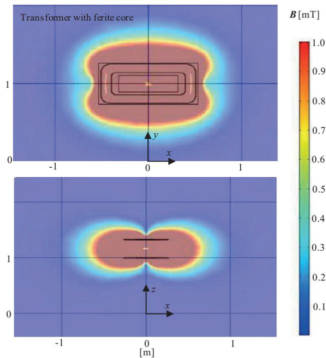
Fig. 7. FEM simulation of magnetic field distribution for coils with ferrite core; current 60 Arms, air gap (distance between coils) 30 cm and frequency 30 kHz. Scale of magnetic field induction in mTrms. a) view in xy-axis, b) view in zy-axis
