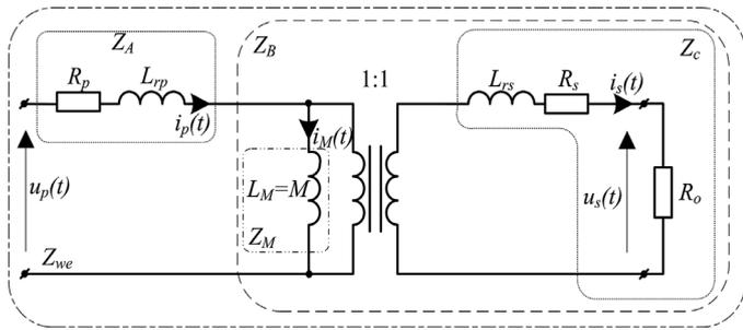
Fig. 2. Transformer equivalent circuit of the IPT system
