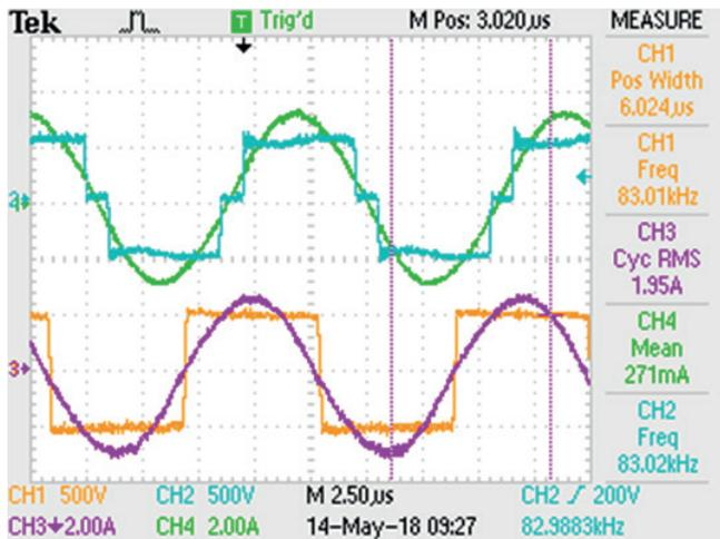
Fig. 13. Experimental results for S-S compensation circuit with constant frequency control (PSM method):  $l = 19$  cm,  $k = 0.12$ ,  $P = 45.6$  kW  $f_{r1} = 83$  kHz ( $i_p$  and  $i_s$  scale x50), ( $u_p$  – CH2 scale x1,  $u_s$  x1, 4 scale x1)
