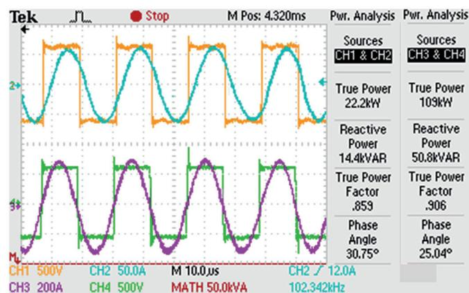
Fig. 11. Currents ( $i_p$  – CH1 scale: x1,  $i_s$  – CH3 scale: /5) and voltages ( $u_p$  – CH2 scale: x1,  $u_s$  – CH3 scale: x1) experimental waveforms in integration method controlled IPT system; magnetic coupling factor  $k = 0.12$ , air gap  $l = 30$  cm, and a resistive load at the power  $P_m = 22$  kW, operating frequency  $f_{r2} = 41.9$  kHz, system efficiency  $h = 92.5\%$
