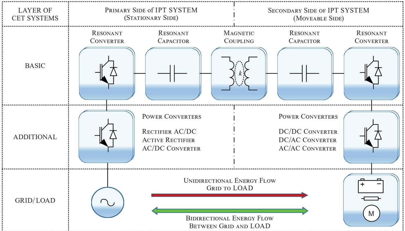
Fig. 1. Functional block diagram of inductive IPT system
