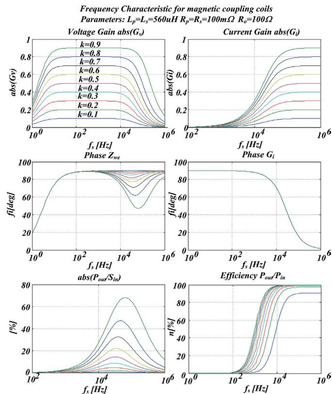
Fig. 3. Frequency characteristics of magnetic coupled coils without compensation circuit
