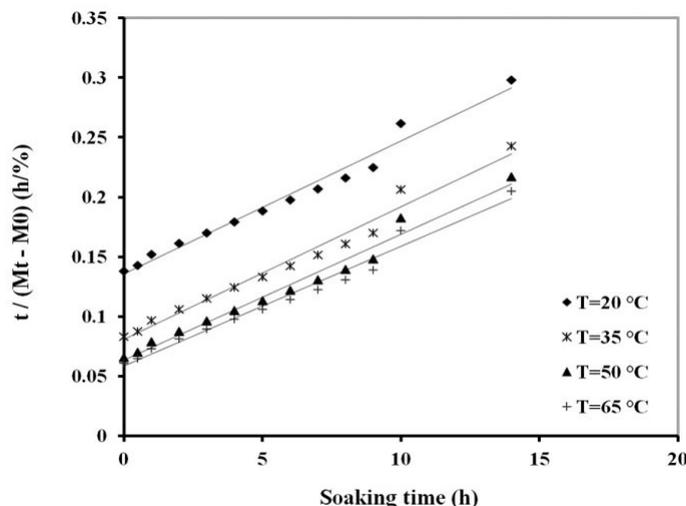
Fig. 5. Fitting of experimental water absorption data of black chickpea to the Peleg's model
