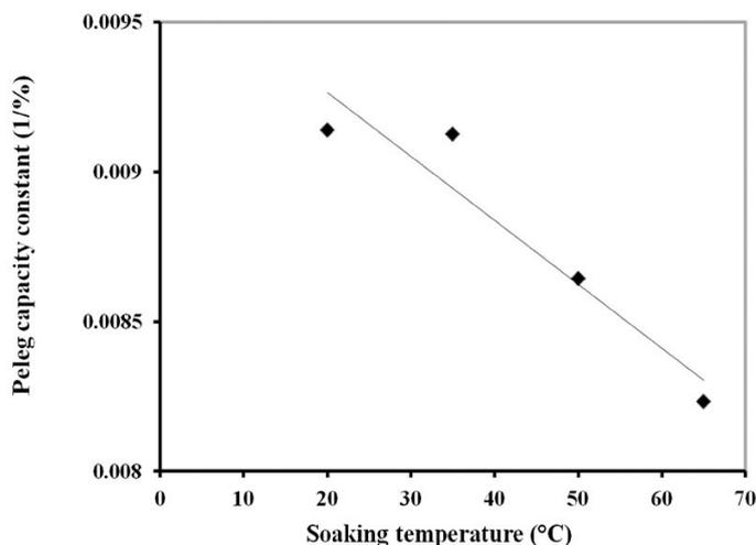
Fig. 6. Effect of medium temperature on Peleg's capacity constant of black chickpea
