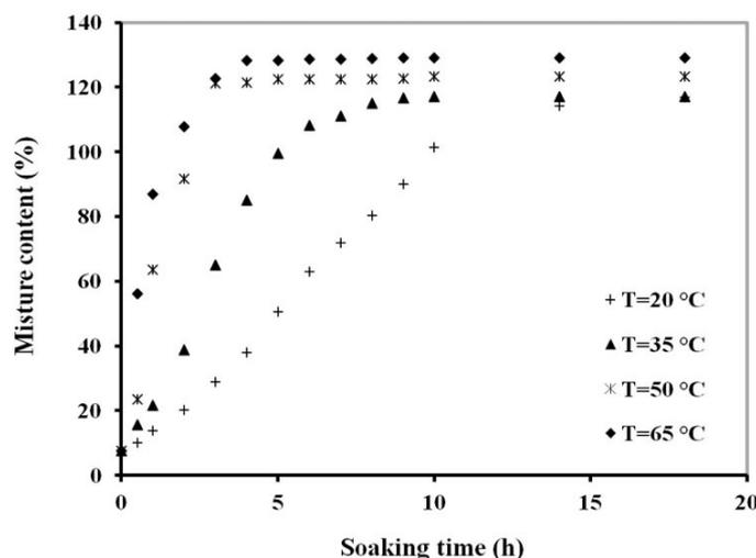
Fig. 2. Hydration of the black chickpea grains at different temperatures between 20 and 65 °C
