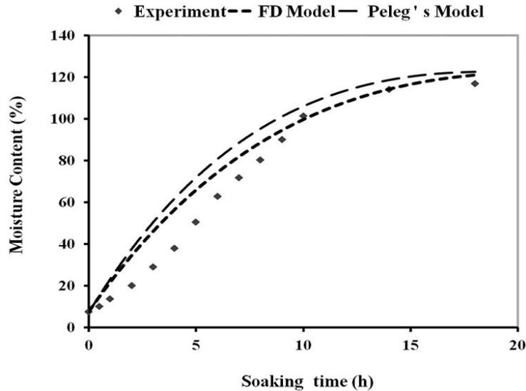
Fig. 7. Comparison of experimental and predicted moisture content of black chickpea obtained in soaking temperature of 20 °C
