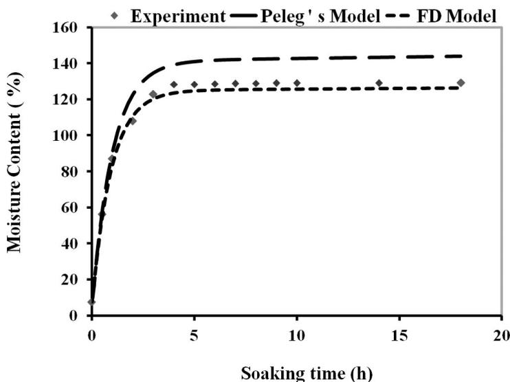
Fig. 10. Comparison of experimental and predicted moisture contents of black chickpea obtained in soaking temperature of 65 °C
