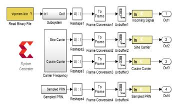
Fig. 2 Input data from MATLAB/SIMULINK to Xilinx System Generator model.
