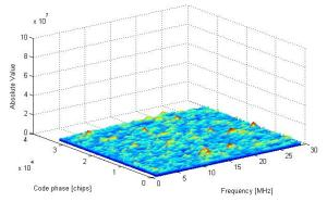
Fig. 8 Acquisition plot for nonvisible satellite.
