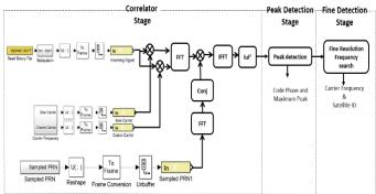
Fig. 1 Block diagram for the Implementation of Acquisition phase in Xilinx System Generator.
