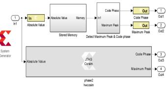
Fig. 6 Implementation of the peak detection stage of acquisition phase using JTAG hardware CO-Simulation.
