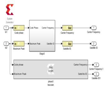
Fig. 9 Implementation of the fine detection stage using JTAG hardware Co-Simulation.
