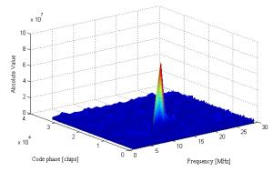
Fig. 7 Acquisition plot for a visible satellite.
