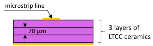
Fig. 5. Cross-section of the designed multilayered microstrip
