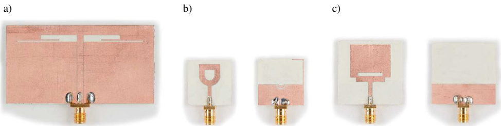
Fig. 4. Photographs of the fabricated prototypes of Antennas I through III optimized using the proposed algorithm: a) Antenna I (gain optimization); b) Antenna II; c) Antenna III.
