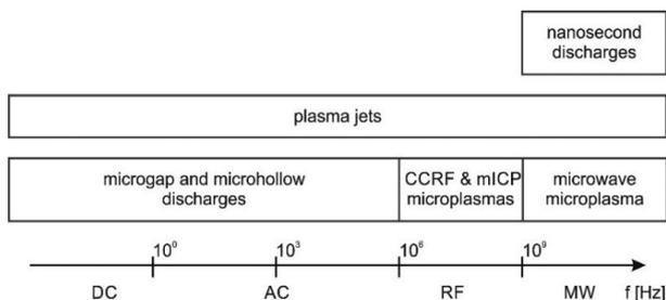
Fig. 2. Classification of micro-plasma sources (based on [11]).
