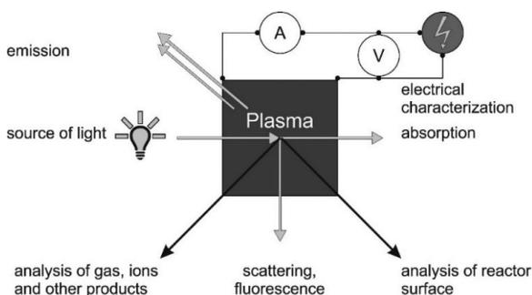
Fig. 3. Methods of micro-plasma characterization (based on [11]).
