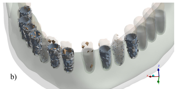
Fig. 2. Statistics (a) and location (b) of poor quality elements (with quality parameter lower than 0.25)
